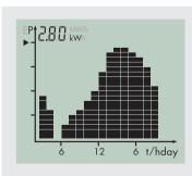
The inverter energy is shown as a diagram on the display. The daily graph is displayed by default. The right-hand flashing bar of the diagram represents the current hour. If the inverter does not feed any power to the grid over a longer period of time (e.g. in darkness or if the PV modules are covered with snow), a gap is inserted into the chart. The bar for the current hour is updated automatically every five seconds.
